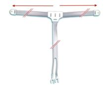
This is a dipole antenna. How long would the "arms" on the wall be (red arrows) if intended as an FM antenna? Hint: dipole antenns are usually design with arm lengths in the order of  $\lambda/4$ .
