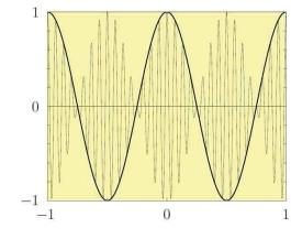
Demodulating AM-SC with an envelope detector:
