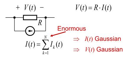
Short pulses, almost unit impulses  $\Rightarrow I(t_1) \& I(t_2)$  almost independent for  $t_1 \neq t_2$
