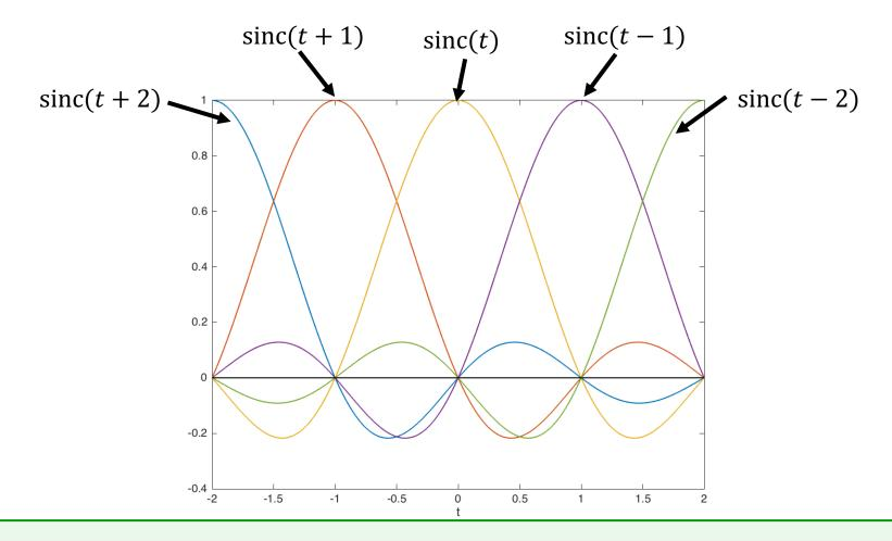
Problems: Non-causal, impossible to implement, sensitive to synchronization errors
