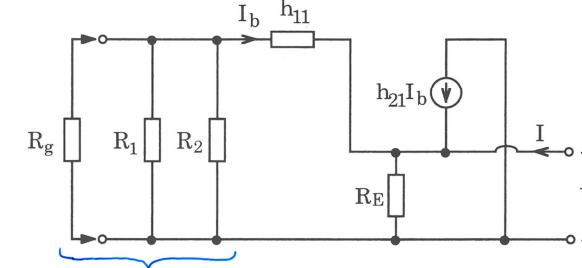
$$\text{Ohms lag: } U = R_E \cdot (I_b + h_{21}I_b + I)$$
