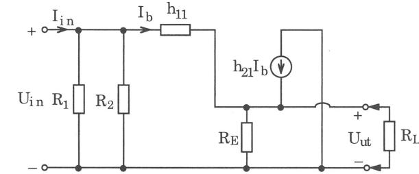
$$\text{KVL: } U_{in} - h_{11}I_b - (R_E \parallel R_L) \cdot (h_{21} + 1)I_b = 0$$
