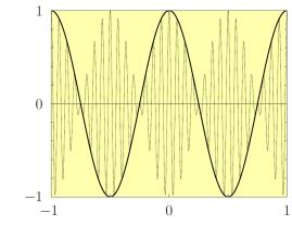
Demodulating AM-SC with an envelope detector:
