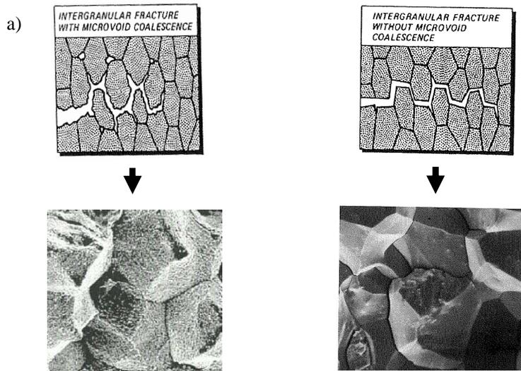
Figure 12 SEM image of intercrystalline fracture a) with microvoid coalescence b) without microvoid coalescence [1].
