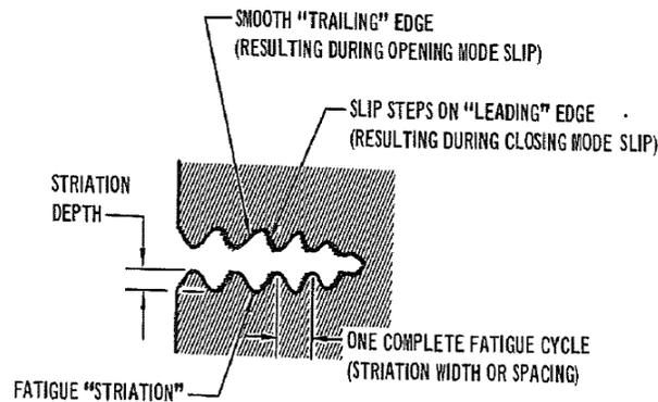
Figure 14 Schematic presentation of formation of fatigue striations.
