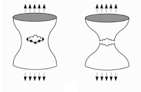
Figure 8 Ductile failure of a metal rod under tensile stress.
