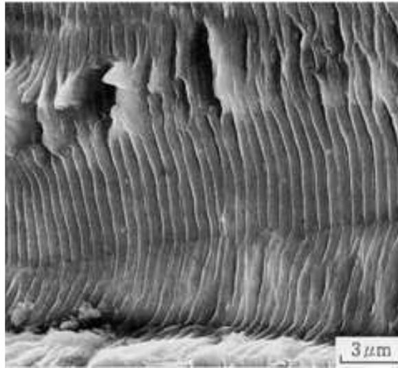
Figure 13 SEM image of fatigue striations. (Can you guess the crack propagation direction?).
