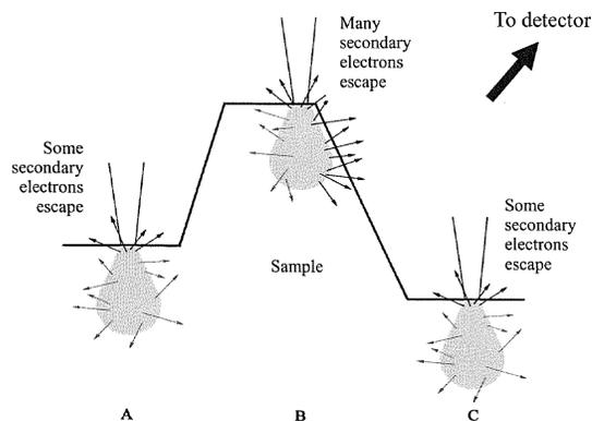
Figure 4 Contrast principle: highest electron yield is gained from protrusions (B), i.e., protrusions appear as bright areas in SEM images.
