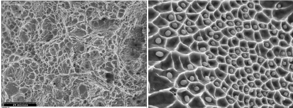
Figure 6 SEM images of a ductile fracture surfaces. Note foreign particles inside the dimples in the right image.
