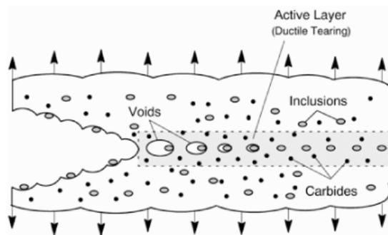
Figure 5 Void nucleation and growth in a ductile material under tensile stress [2].
