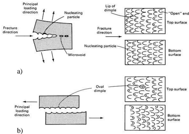
Figure 7 Examples of ductile fractures with varying dimple shapes. a) Tearing produces elongated dimples on both fracture surfaces that point back to the crack origin; b) shear stresses generate dimples elongated in the shearing direction [3].
