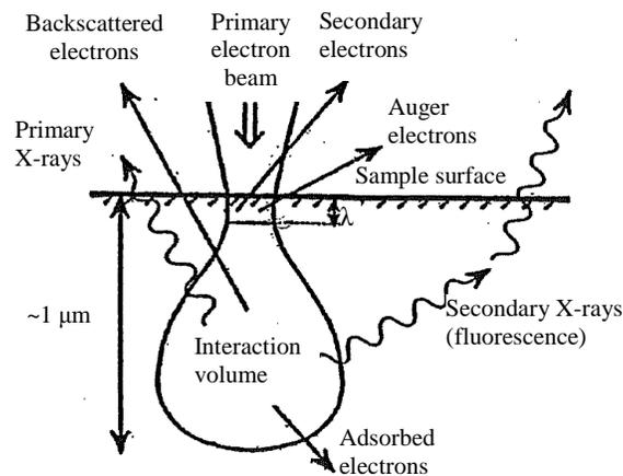
Figure 3 Electron beam – sample interaction ( $\lambda$  – electron mean free path).
