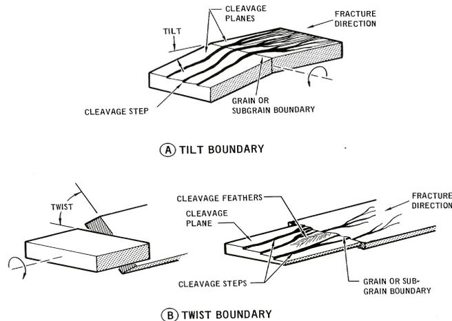
Figure 11 Cleavage fracture: a) crack propagation direction changes at tilt boundary; b) branches of river pattern originate at twist boundary [3].
