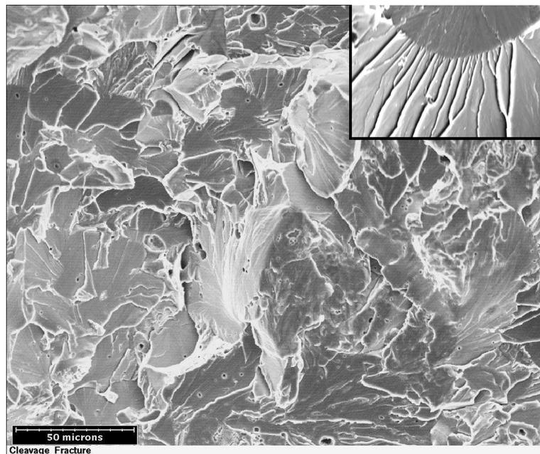
Figure 10 SEM image of a cleavage fracture. The inset shows a twist boundary at higher magnification.
