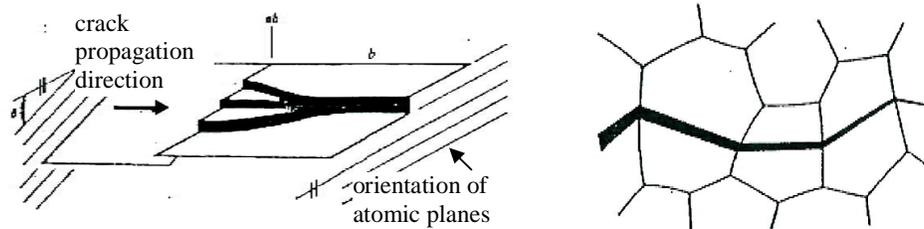
Figure 9 a) Height of the cleavage step increases along crack propagation direction; b) a crack propagates through a polycrystalline material (transcrystalline fracture), from left to right. The crack changes direction locally as it passes each grain boundary [3].
