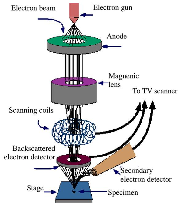
Figure 2 Schematic illustration of a scanning electron microscope (SEM).
