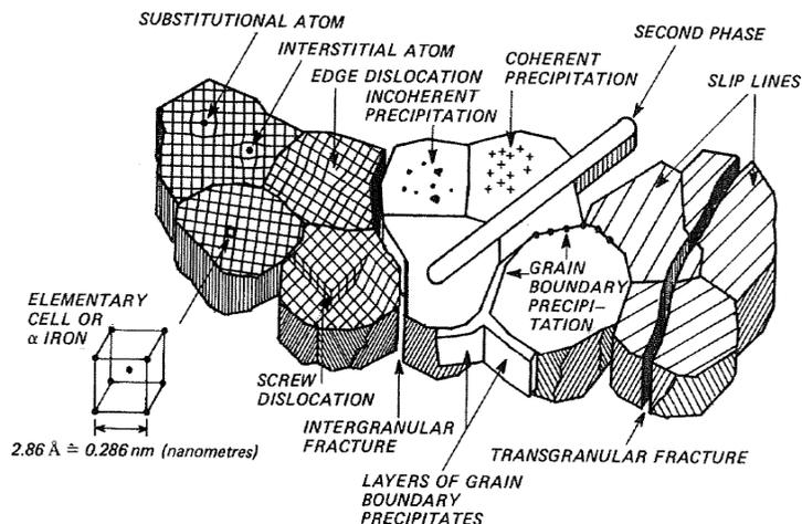
Figure 1 Schematic of microstructural features in metallic materials [1].
